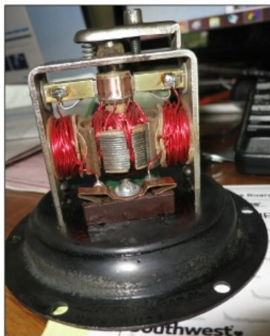
Rewound field and armature by Steve Smith
